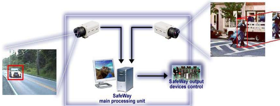
Figure 1. Basic SafeWay configuration: one IBM-PC compatible computer, two video surveillance cameras and one device for other equipment interfacing to the system
